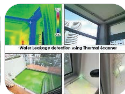
Ponding Test & Water Leakage detection
